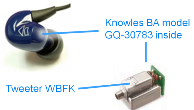
Figure 3: Example Knowles reference design earphone with BA meeting Hi-Res Audio requirements.
