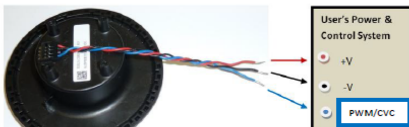
Figure 10. SynJet Power and Control Electrical Interface to User System
