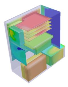
A CFD analysis shows how system level design is paramount for optimizing product performance and packaging since considerable heat needs to be removed from the air stream for 64 bit processors.
