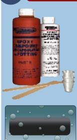
Epoxies are two part encapsulating compounds. They are mixed and then poured onto the circuit board. Once cured, the result is extremely hard and durable. Epoxy is most effective when board is cover with at least <sup>1</sup>/<sub>4</sub> inch in thickness. Epoxies provide
