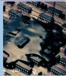
excellent protection against impact, shock, conductivity, moisture, abuse, chemicals, and analysis. Provides technology security. Excellent for explosion proof components. Epoxies are extremely difficult to remove.
