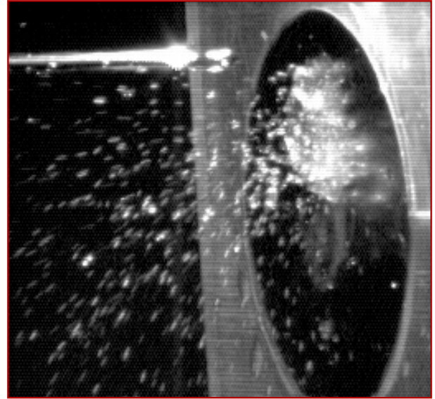
Figure 10a. Ejected secondary droplets with the atomizer in a vertical orientation. The supply tube is normal to the atomizer.
