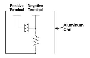
The dummy terminal(s) of a non-solid capacitor are not internally insulated from the negative terminal (cathode) due to an indeterminate resistance caused by an electrolyte coating on the terminals inside the can.
