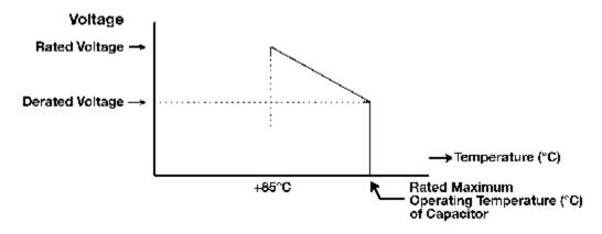
Using a voltage greater than the derated voltage will damage the dielectric of a capacitor.
