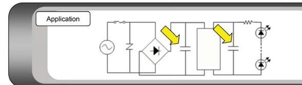
Best for LED lighting's smoothing circuit, noise absorption, LED protection thanks to large capacitance.
