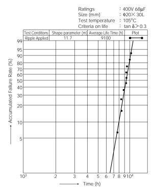
Fig. 2-12 Failure Analysis by Weibull Probability Paper
