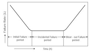
Fig. 2 - 11 Failure Rate Curve (Bathtub Curve)
