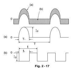
Setting Model 2 as the ripple current for a low frequency component (IL):
