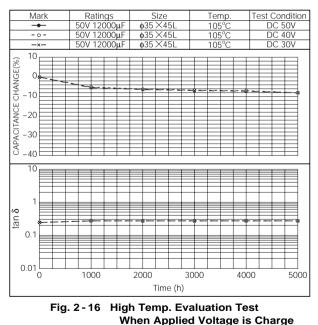
In regards to high voltage capacitors used in smoothing circuits for power electronic equipment, the leakage current decreases as the voltage drops and lessens the consumption of electrolyte. In such cases, the life of the capacitor may be extended. For more details, please contact our sales offices.
