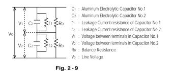
If the leakage current of  $C_1$  and  $C_2$  are expressed as  $i_1$  and  $i_2$  :
