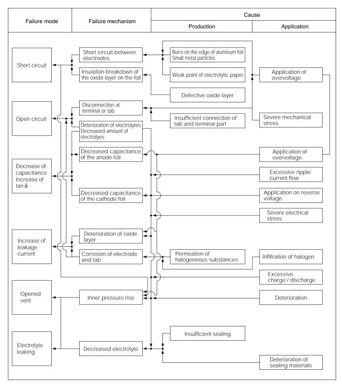
Fig. 2-1 Analysis of Failure Mode
