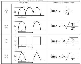
Effective ripple value is calculated from the wave form of ripple, which ripple current of high frequency switching (I<sub>H</sub>) is superposed upon ripple current of commercial frequency (I<sub>L</sub>)(as in Figure 2-17), by dividing it into each frequency component.
