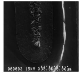
Photo 1-4 Enlarged photo of middle, high voltage formed foil. (Condition of oxide layer formation in a pit)
