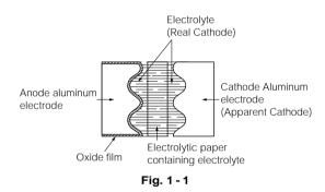
Since the oxide film has rectifying properties, a capacitor has polarity. If both the anode and cathode foils have an oxide film, the capacitors would be bipolar (non-pola) type capacitor.
