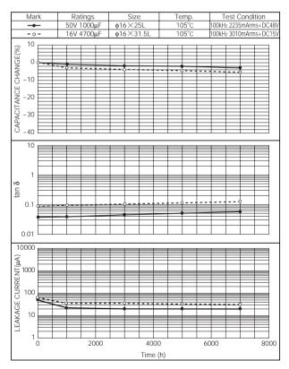
Fig. 2 - 14 High Temperature Life Evaluation Test
