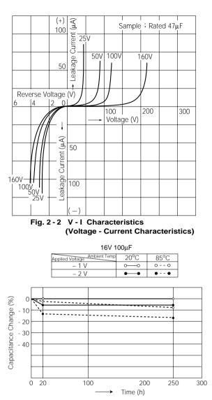
Fig. 2-3 Capacitance vs. Reverse Voltage Characteristics
