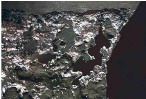
Iron erosion of stainless steel pot material
