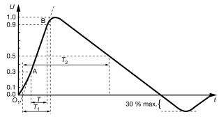
Front time:  $T_1 = 1.67 \text{ x } T = 1.2 \text{ } \mu\text{s} \pm 30 \text{ } \%$ Time to half-value:  $T_2 = 50 \text{ } \mu\text{s} \pm 20 \text{ } \%$
