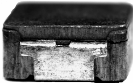
Terminal area crack, acceptable
