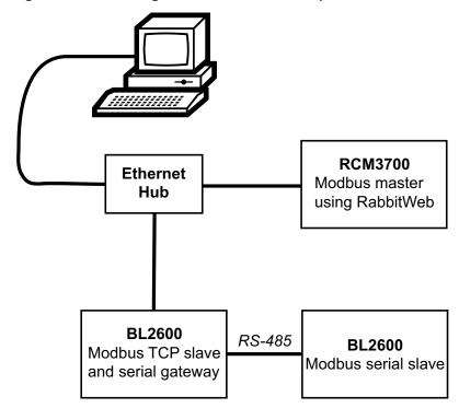
Figure 1. Test Configuration Used to Develop Modbus Libraries
