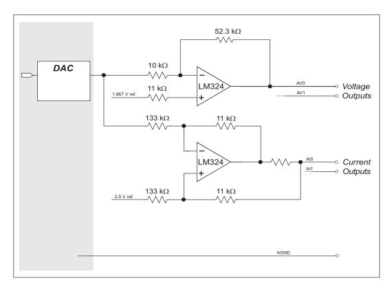
Figure 8. Buffering and Scaling D/A Converter Outputs
