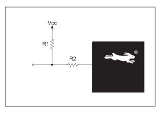
Figure 1. Pulled-Up Input
