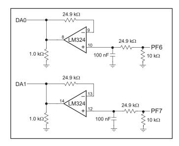
Figure 3. Schematic Diagram of D/A Converters
