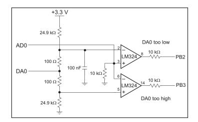
Figure 6. Discrete Inexpensive Op-Amp Based A/D Converter
