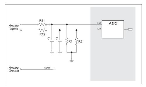
Figure 7. Resistor Divider Network to Filter and Scale Analog Inputs
