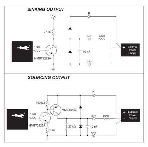
Figure 10. Sinking and Sourcing Digital Outputs
