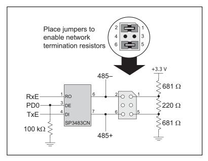
Figure 4. Sample Motherboard RS-485 Interface Circuit
