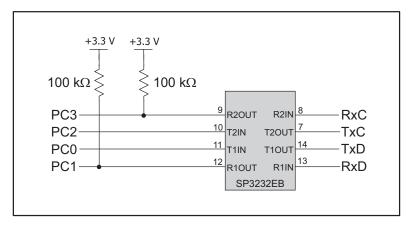
Figure 5. Sample Motherboard RS-232 Interface Circuit
