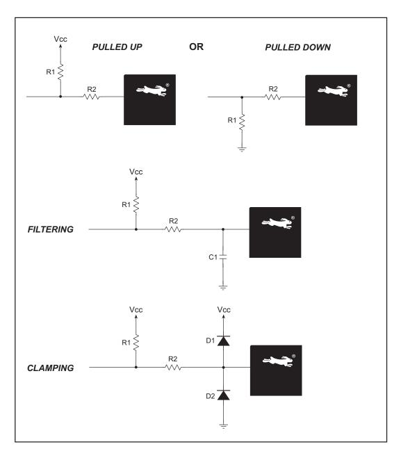
Figure 9. Digital Input Setup
