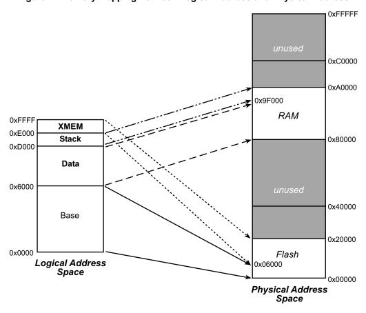
Figure 1. Memory Mapping Between Logical Address and Physical Address
