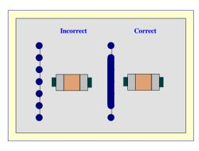
Using a slot along the depanelisation edge reduces the level of stress exerted onto the capacitor by approximately 50%.
