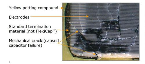
Black areas are damaged sections within the capacitor caused during the electrical failure
