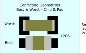
Reducing the pad/ land size can reduce the level of stress exerted onto the capacitor by approximately 50%.
