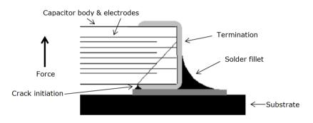
Figure 1: Mechanical Crack
