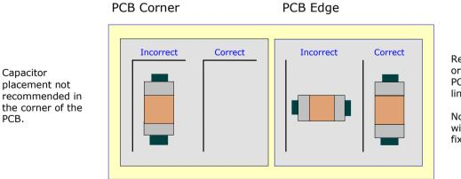
Recommended capacitor orientation with respect to PCB edge (denoted by black lines).
