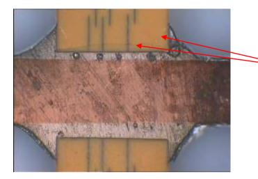
Fig 14 Example of force cooled 99.3Sn/0.7Cu solder joint showing longbow and corner cracks
