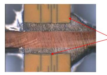
Fig 13 Example of 60Sn/40Pb solder joint showing longbow and corner cracks
