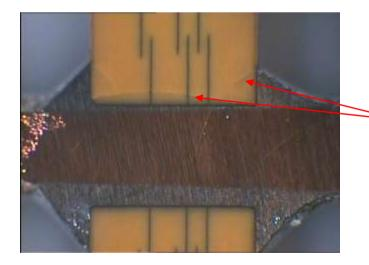
Fig 17 Example of 95.5Sn/3.8Ag/0.7Cu solder joint showing longbow and corner cracks
