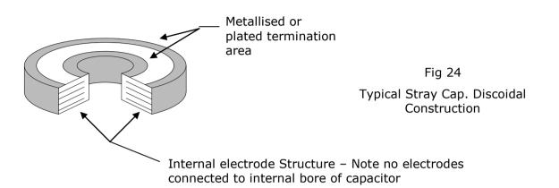
The capacitance is created by the interaction of the internal bore termination and the outer earth electrodes.
