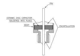
Fig 3 Typical Emi Filter Construction
