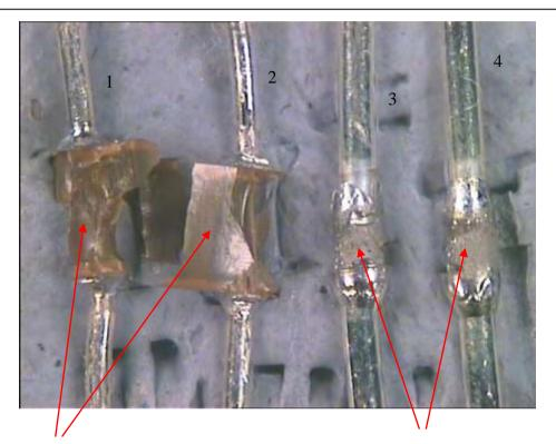
Fractured ceramic remaining attached to the feedthrough pin after attempting to pull the pin out.
