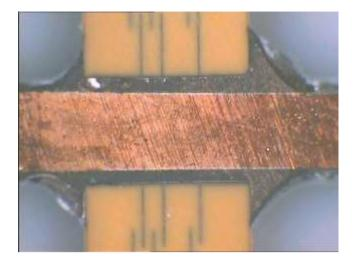
Fig 18 Example of force cooled 50Pb/50In solder joint showing absence of any cracks
