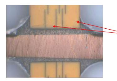
Fig 12 Example of force cooled 60Sn/40Pb solder joint showing longbow and corner cracks
