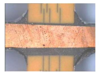
Fig 19 Example of 50Pb/50In solder joint showing absence of any cracks
