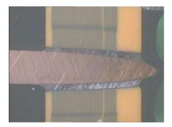
Fig 21 Example of 95Pb/5In solder joint showing absence of any cracks
