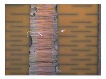
Fig 31 Further example of leaching and poor solder joint with PdAg termination.
