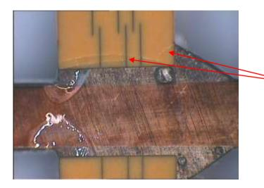
Fig 15 Example of 99.3Sn/0.7Cu solder joint showing longbow and corner cracks
