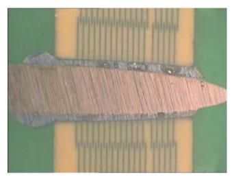
Fig 20 Example of force cooled 95Pb/5In solder joint showing absence of any cracks
