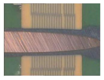
Fig 23 Example of 93.5Pb/5Sn/1.5Ag solder joint showing absence of any cracks
