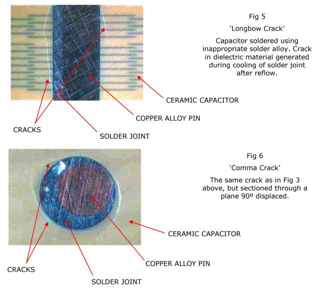
Cracks in the dielectric material can result in catastrophic electrical breakdown of the capacitor if they propagate through the active electrode area. Cracks are considered quality defects and cannot be accepted for high performance applications.
