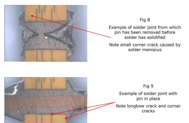
This showed that the cracks only occur during the cooling portion of the soldering profile, and that pins must be present to generate the forces that form the longbow crack. This shows that the forces exerted on the ceramic are external to the capacitor.
