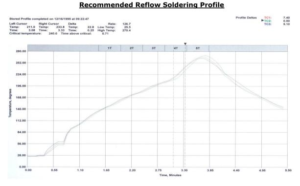
When discussing a reflow profile, we can only give a general recommendation as to the shape of the profile. We cannot give a definitive profile of the actual peak temperatures, as this is dependant on a number of factors which can only be decided by the assembler – the type of solder used, the size, specification and arrangement of other components on the board and the overall thermal mass of the board.
