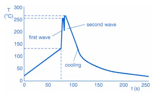
Maximum permissible wave temperature is 270°C for SM chips and 260°C for Radial Leaded capacitors – see also note above regarding radial leaded capacitors.
