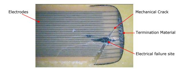
Mechanical cracking always initiates from the point of highest stress, which is at the junction of the ceramic body and the termination band.
