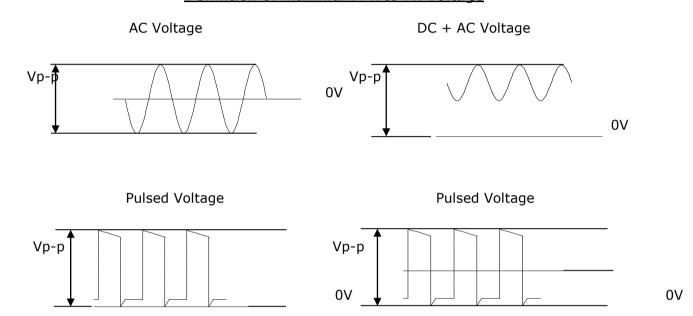
The rated peak to peak voltage of 600 volts should not be exceeded in each of the above options.
