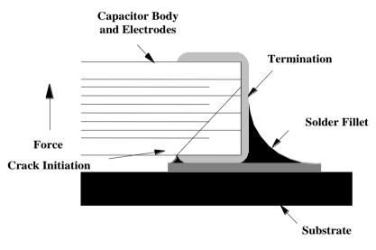
Fig 1. Mechanical Crack
