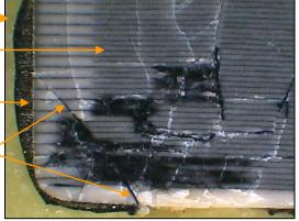
Black areas are damaged sections within the capacitor caused during the electrical failure
