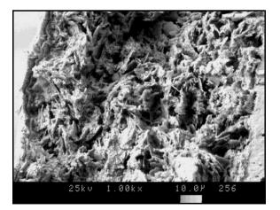
Picture taken at 1000x magnification using a SEM showing a fracture section through a capacitor termination.
