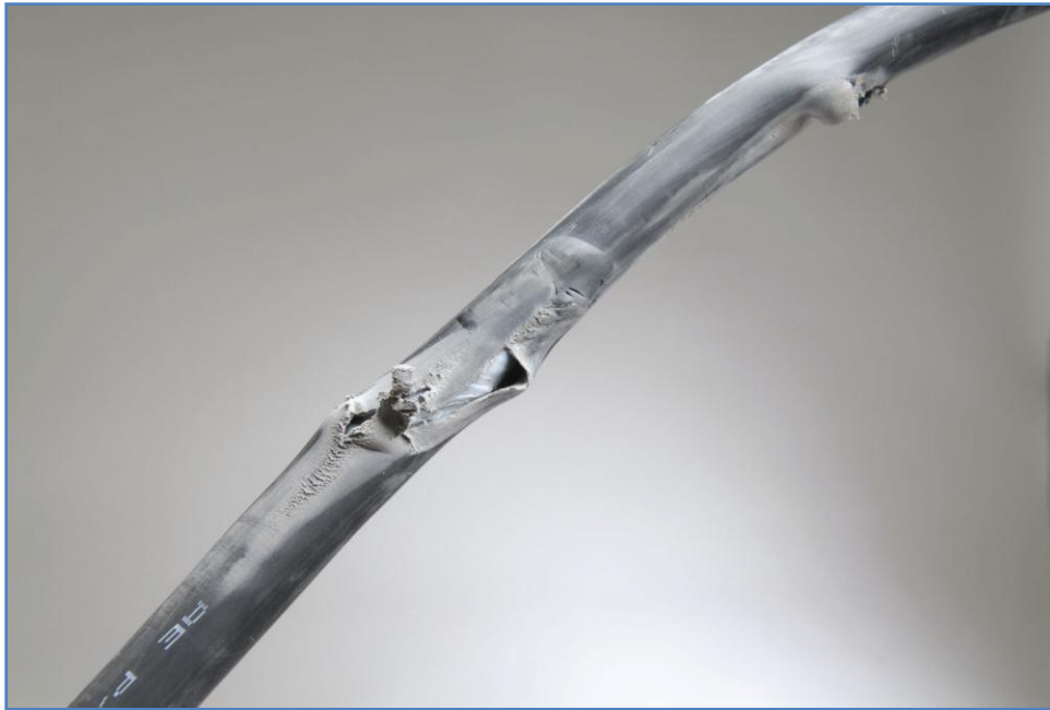
Figure 2. Heat-shrink tubing can be used to repair worn and damaged wire and cable.
