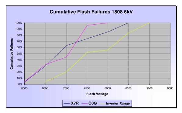
Results show a significant improvement in performance over Syfer standard high voltage components manufactured from both X7R and C0G materials, arcing inception is increased by 500V to 6.5kV and ultimate performance is improved by up to 1kV.
