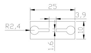
Above: Test Board and Dimensions (mm)
