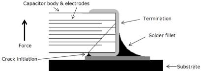
During Syfer's initial investigation into mechanical cracking over 15000 capacitors were subjected to bend testing.
