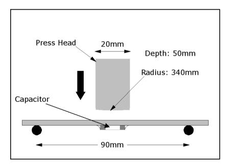
Fig 1. Bend Test Method
