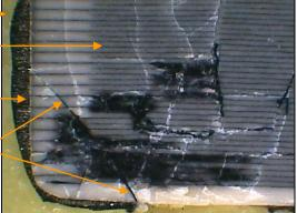
Black areas are damaged sections within the capacitor caused during the electrical failure
