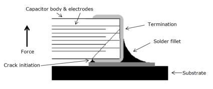
Fig 1. Mechanical Crack
