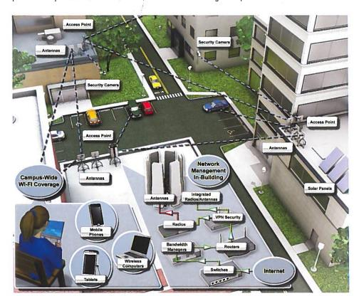
With a standard in-building DAS, the cellular source, such as a wireless base station, provides the wireless signal to the building through an antenna or wired land-line connection. In the building itself, the DAS consists of headend equipment, bi-directional amplifiers, fiber distribution remote units, and in-building antenna access points - all of which may be connected through Carol's DBRF Flexible Low Loss Coaxial Cables and General Cable's NextGen® Brand fiber optic cables.
