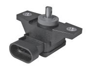
Round and round the globe, it's Honeywell. So trust Honeywell Sensing and Control (S&C) for your Hall-effect rotary position sensor needs. These transducers vary output voltage or current in response to changes in a magnetic field — using a magnetically biased Hall-effect integrated circuit (IC) to sense rotary movement of the actuator shaft. The rotation of the shaft changes the IC's position to the magnets, and then detects the
