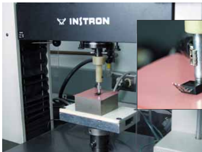
Cut-Through Resistance - Bergquist introduced its TO-220 cut-through test to help customers better understand typical application performance.
