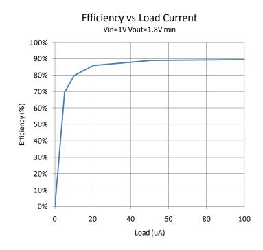
Figure 2: The ultra low-power op amp based charge-pump boost converter exhibits 90% efficiency over a wide range of load currents.
