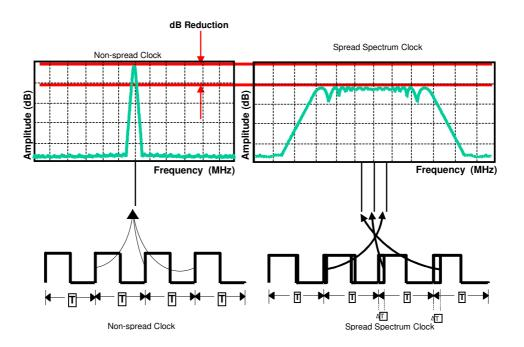
Figure 2. Spectrum plots of a non-spreading clock and a spread spectrum clock as measured by a spectrum analyzer with a 100 KHz resolution bandwidth
