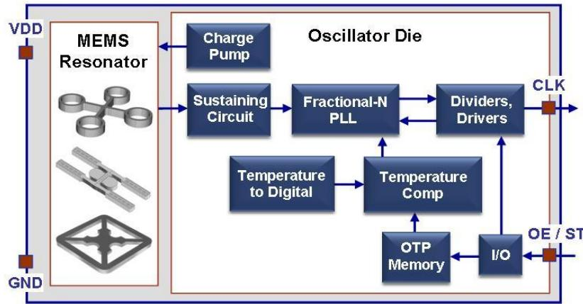
Figure 1: Programmable architecture of SiTime's MEMS-based oscillators
