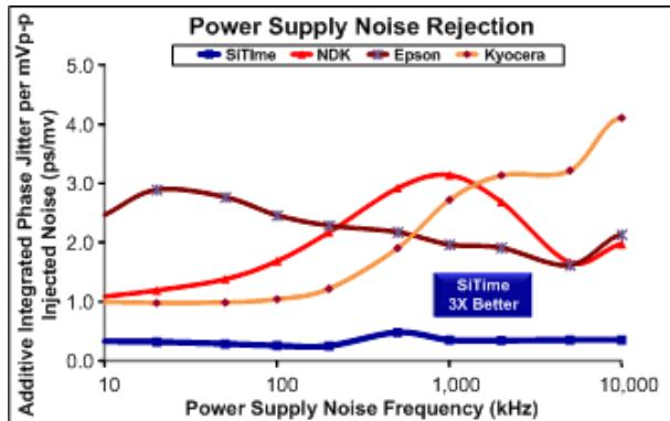
Figure 6: Power Supply Noise Rejection [5]
