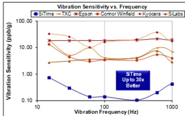
Figure 7: Vibration Robustness [6]
