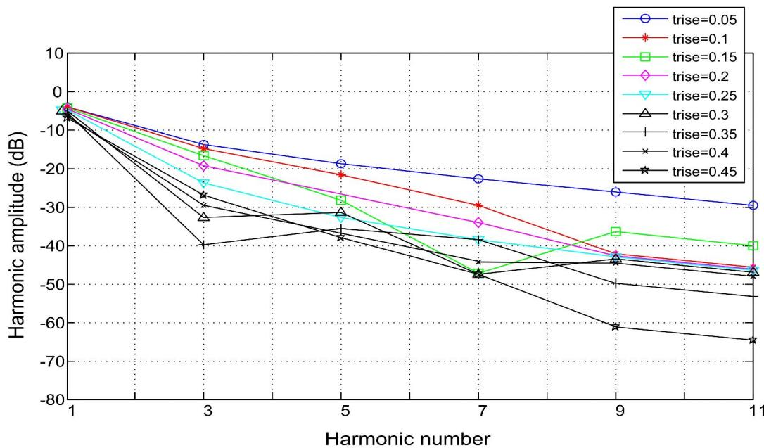
**Figure 3: Harmonic EMI reduction as a function of slower rise/fall time**
