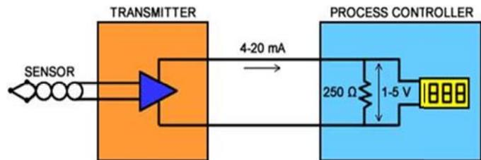
The precision resistor converts the 4-20 mA signal from the transmitter to a voltage drop, which is compatible with the data processing components. Normally, the resistor is contained in the input circuitry of the data processing equipment.
