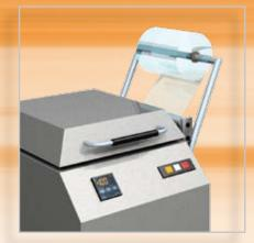
Sealing Clear indication that the correct temperature has been reached thanks to the deviation indicator.
