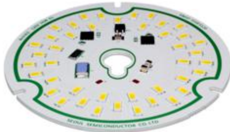
Seoul Semiconductor Acrich2-- a 120V, 16W AC LED Module
