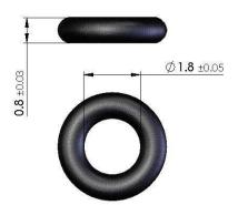
O-Ring receptacle cylinder sizes and tolerances used in the evaluation assembly.
