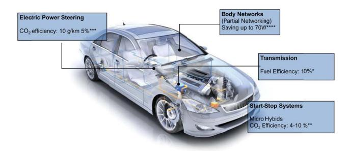
In summary, the potential efficiency gains for the systems just mentioned are: Start/stop systems will reduce fuel consumption and  $CO_2$  emissions between 4% and 10%; electric power steering can save 10 g/km in  $CO_2$  emissions; dual-clutch systems deliver 10% energy savings compared to conventional five-speed automatic transmissions; and, partial body networks can save up to 70W.
