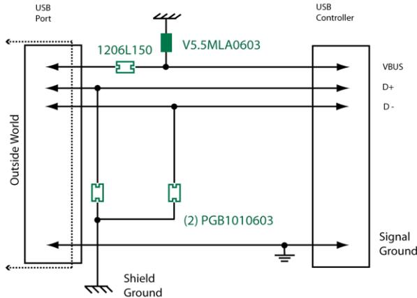
Possible solution: D+/D-: PGB102ST23 polymeric suppressor (0.05 pF)
