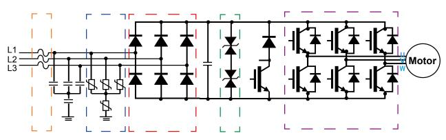
Figure 1: Typical three-phase VFD/Inverter topology with protection components
