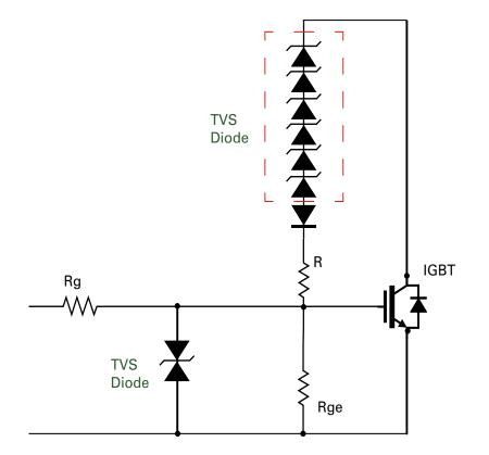
Figure 4: Active clamping function
