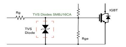
Figure 3: IGBT gate protection
