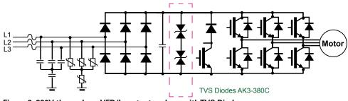
Figure 2: 380V three-phase VFD/Inverter topology with TVS Diodes
