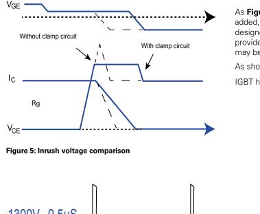
As **Figure 5** illustrates, with active clamping circuit added, the  $V_{CE}$  inrush voltage is reduced. But how can a designer calculate the number of TVS Diodes needed to provide such inrush protection? The following example may be useful for reference.
