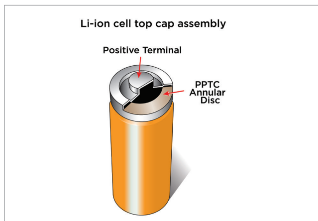
Figure 8. A PolySwitch disc device's placement on an 18650 battery cell.
