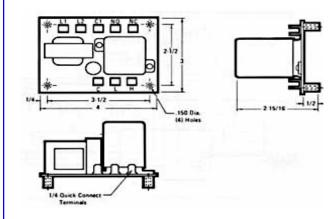
This is a fixed-sensitivity, forward mode control. The control relay is energized when liquid rises to contact the "H" probe. The control relay is pulled in and remains energized until liquid drops below the "L" probe.
