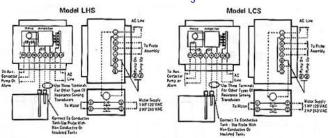
Models LCS/LHS is a forward mode control. The control relay is energized when liquid rises to contact the "H" probe. The control relay is pulled in and remains energized until liquid drops below the "L" probe. Sensitivity is adjustable.
