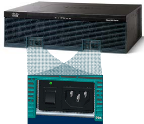
Figure 1: Integrated Services Router AC power input module. Optional DC wiring module was required to mount in same available space.
