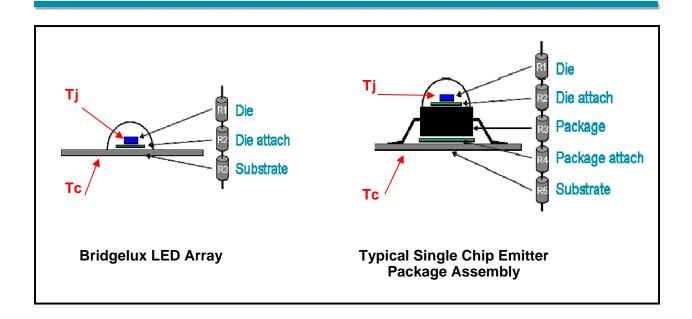
Fig 1: Comparison of thermal path for Bridgelux LED Array and a typical single chip emitter package
