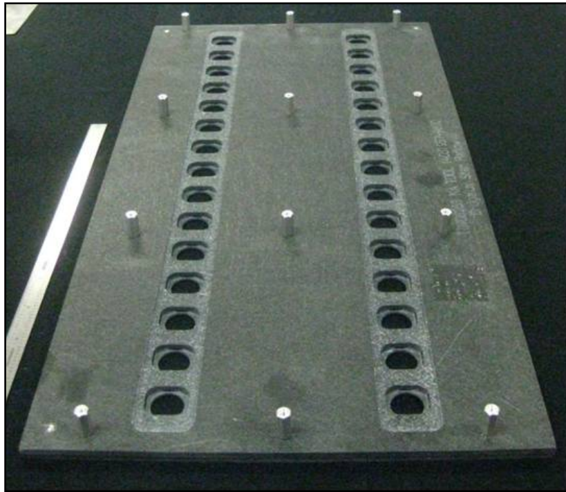
Figure 16: Solder reflow fixture for Rectangular LED Arrays with both plates clamped together using screws
