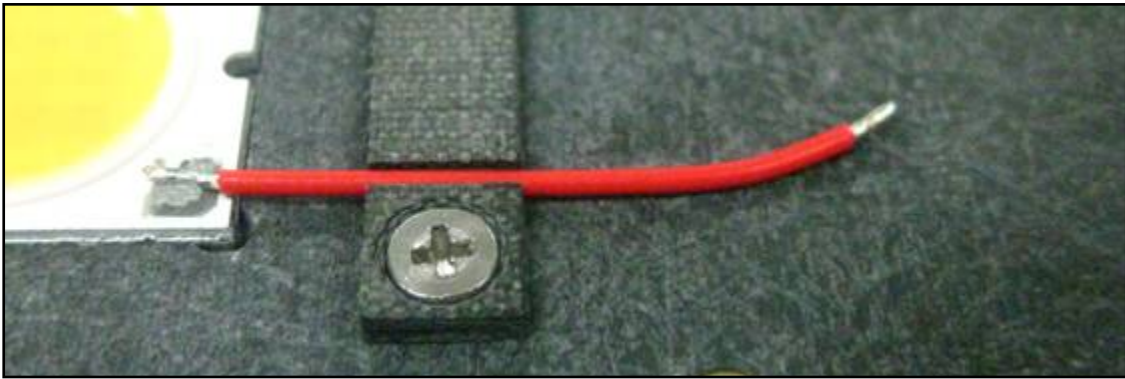
Figure 12: Wires from spools with curvature must lay flat on the fixture
