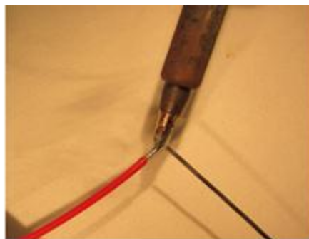
Figure 11a: Pre-tin the wire using a soldering iron
