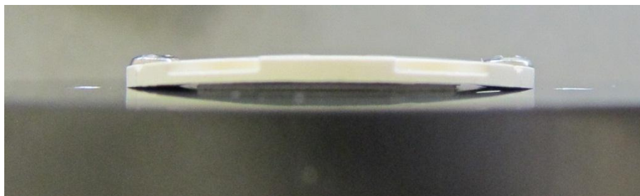
Figure 18: Typical Flex of Vero LED Module
