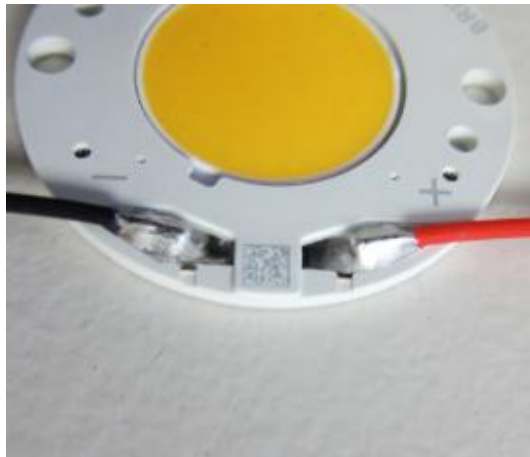
Figure 14: Good solder joints
