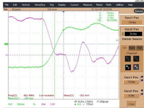
FIGURE 8. Measured current and voltage turn-on switching transient.
