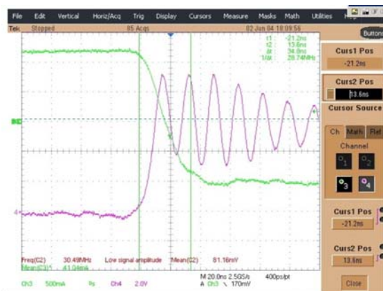
FIGURE 9. Measured current and voltage turn-off switching transient.
