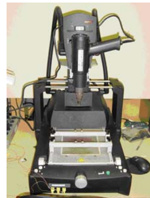
Figure 7. Mechanical fixture to hold the heat gun
