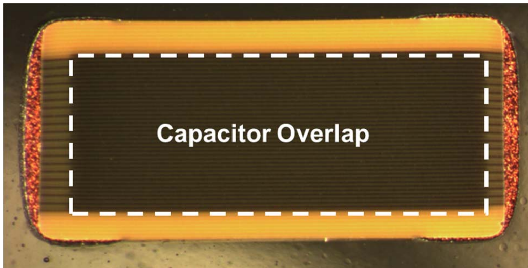
Figure 1. Cross-section of a standard 200VDC rated X7R MLCC
