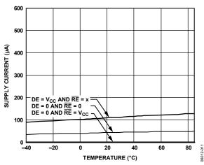
Figure 11. ADM483E Supply Current vs. Temperature
