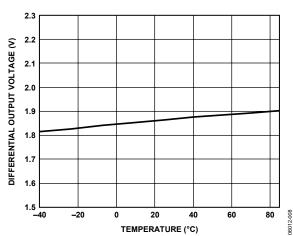
Figure 8. Driver Differential Output Voltage vs. Temperature
