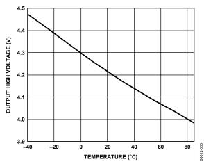
Figure 5. Receiver Output High Voltage vs. Temperature
