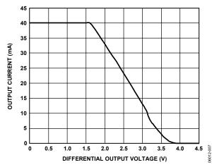
Figure 7. Driver Output Current vs. Differential Output Voltage
