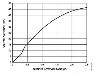
Figure 3. Output Current vs. Receiver Output Low Voltage
