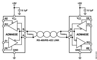
Figure 23. Typical Half-Duplex Link Application
