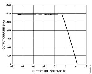
Figure 10. Output Current vs. Driver Output High Voltage
