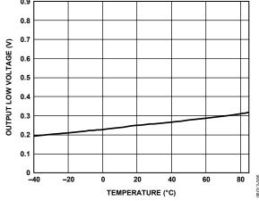
Figure 6. Receiver Output Low Voltage vs. Temperature
