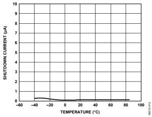
Figure 12. Shutdown Current vs. Temperature
