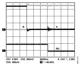
Figure 14. ADM483E Receiver t<sub>PLH</sub> Driven by External RS-485 Device
