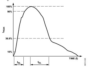
Figure 25. Human Body Model ESD Current Waveform
