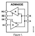
Drivers are short-circuit current-limited and are protected against excessive power dissipation by thermal shutdown circuitry that places their outputs into a high impedance state. The receiver input has a fail-safe feature that guarantees a logic high output if the input is open circuit.
