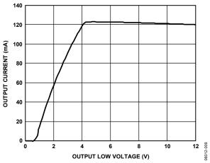
Figure 9. Output Current vs. Driver Output Low Voltage
