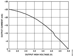
Figure 4. Output Current vs. Receiver Output High Voltage
