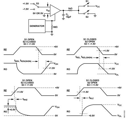
Figure 22. Receiver Enable and Disable Times
