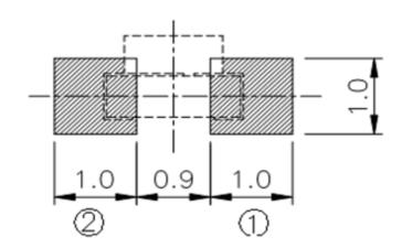
For Reflow Soldering (propose)
