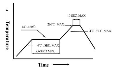
3). DIP soldering (Wave Soldering):
